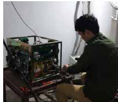
Fig 3: Repairing x-ray generator in jaubari PHC of Gorkha Workshop.
