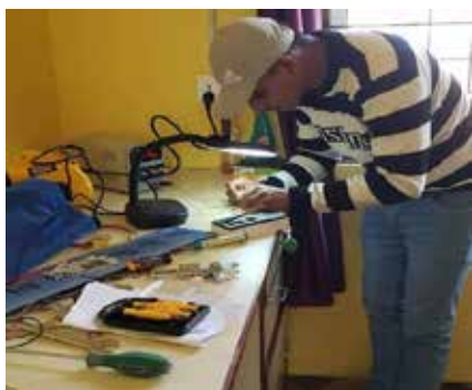
Fig 2: Repairing power board of baby warmer in parbat district hospital.
